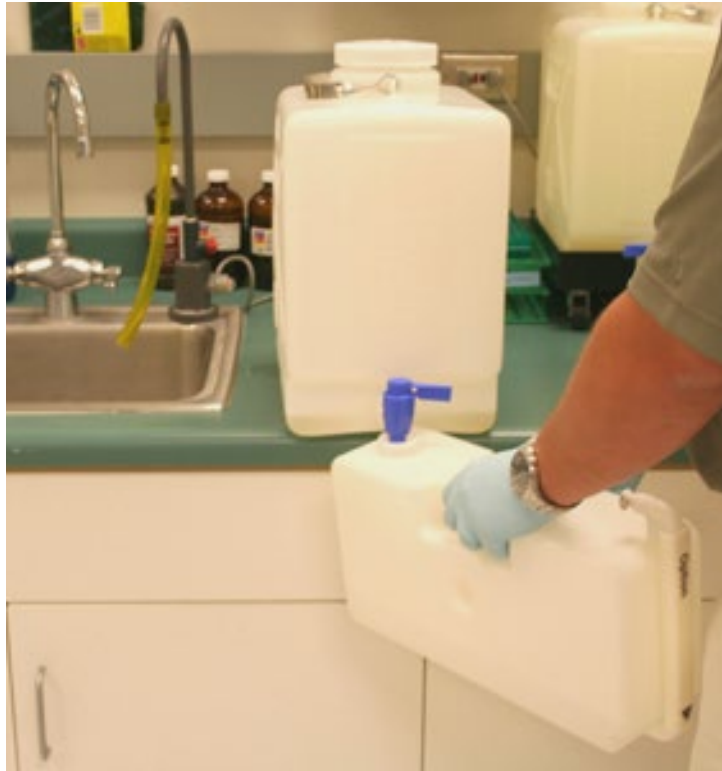
Figure 227. Refilling Bulk Fluid Bottles with Fresh Bulk Fluids
