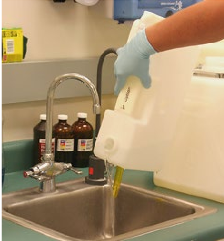
Figure 226. Emptying Residual Fluids from Bulk Fluid Bottles
