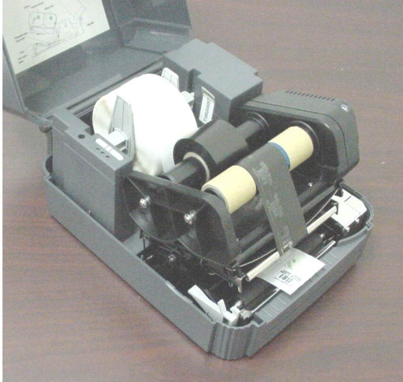
Figure 272. Installation of Label Stock and Thermal Transfer Ribbon
