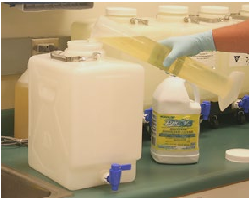
Figure 225. Placing Disinfectant Solution in Carboy
