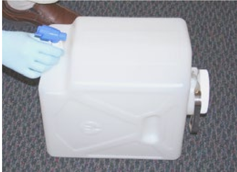
Figure 66. Spigot Placed on Threaded Connector
