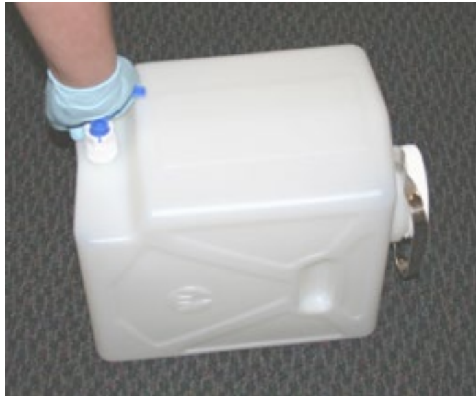
Figure 67. Tightening the Spigot's Locknut
