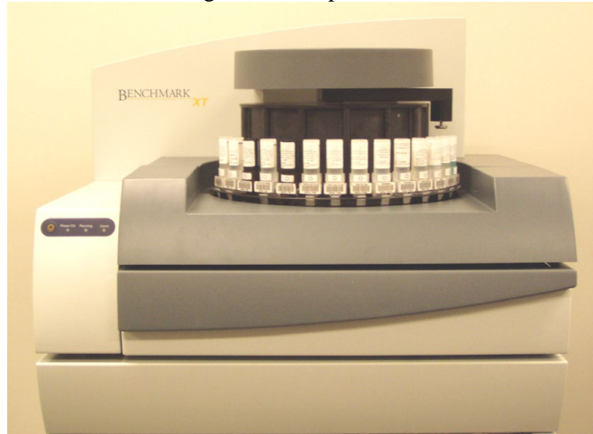
Figure 17. Stainer Subassembly
