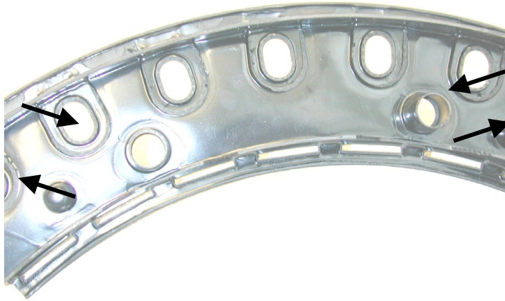
Figure 34. Steel Inserts and Mounting Holes in Bottom of Reagent Tray
